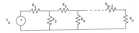
Let n=8,  $R_1=R_3=R_5=R_7=3\Omega$ ,  $R_2=R_4=R_6=R_8=1\Omega$ . Calculate the voltages and currents for  $V_g=1V$  using the program written.
