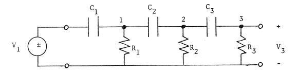
Find  $V_3/V_1$  for this circuit at  $\omega$  = 2 rad/sec in the following ways, comparing the effort required. Take  $R_1$  =  $R_2$  =  $R_3$  =  $2\Omega$ ,  $C_1$  =  $C_2$  =  $C_3$  = 1F.
