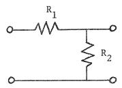
The transfer function  $\frac{R_2}{R_1+R_2}$  must lie between 0.46 and 0.53. The input resistance  $R_1+R_2$  must lie between 1.85 and 2.15. Optimize the tolerances  $\epsilon_1$  and  $\epsilon_2$  on  $R_1$  and  $R_2$ , respectively, and find the best corresponding nominal values  $R_1^{\ 0}$  and  $R_2^{\ 0}$  using the following cost functions:
