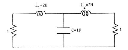
Obtain the partial derivative values of the insertion loss in dB of the filter between the terminating resistors with respect to  $L_1$ , C and  $L_2$  using the adjoint network method. If  $L_1$  changes by +5%,  $L_2$  by -5% and C by +10%, estimate the change in insertion loss at  $\omega$  = 1 rad/sec. Check your results by calculating the change in loss directly and explain any discrepancies.
