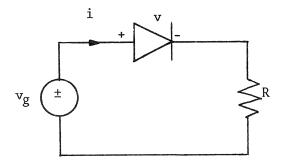
illustrate with the aid of an i-v diagram an iterative method of finding v at d.c. State Newton's method for solving this problem and derive the network model corresponding to the situation at the jth iteration. What is the significance of this model?
