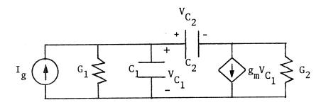
Derive from first principles the adjoint network and sensitivity expressions for all the elements of the circuit. Derive the adjoint excitations appropriate for calculating the first-order sensitivities of  $V_{\text{C}_2}$  w.r.t. all the parameters.
