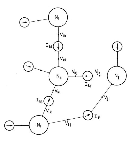
Fig. 2 Network blocks with added current sources.
