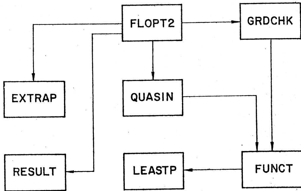
Fig. 1 Overall structure of FLOPT2.
