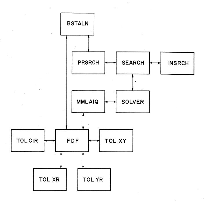
Fig. 8 Structure of the program for the best alignment problem.
