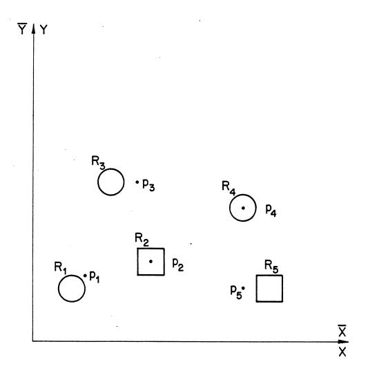
Fig. 9 Points and tolerance regions before alignment.
