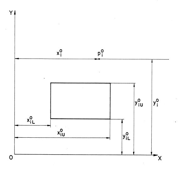
Fig. 5 Regular point with the rectangular tolerance region.
