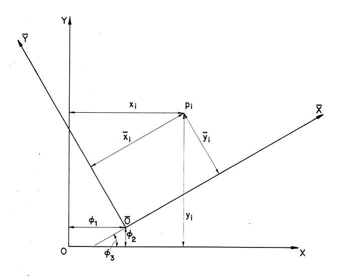
Fig. 3 Transformation of coordinates relating the two systems of coordinates.
