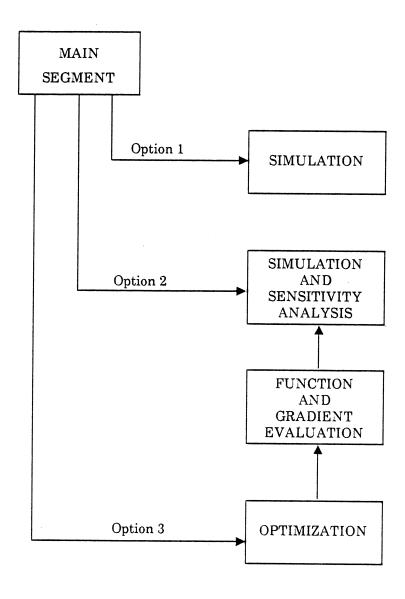
Fig. 1 Functional blocks of the computer package for multiplexer simulation, sensitivity analysis and optimization.
