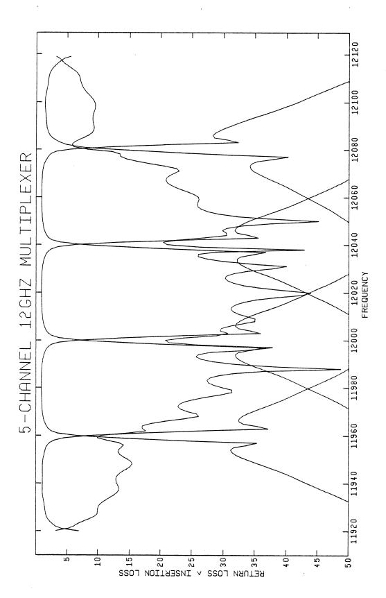
Responses in dB of a 5-channel multiplexer (including two dummy channels) with optimized spacings and input-output transformer ratios. The filters are lossy and dispersive with unloaded  $\mathbf{Q}=12000$ ; nonideal junctions are assumed. Fig. 2
