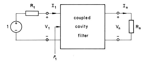
Fig. 1 Doubly terminated multi-coupled cavity microwave filter.
