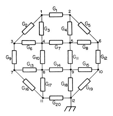
Fig. 4 The resistive mesh network.
