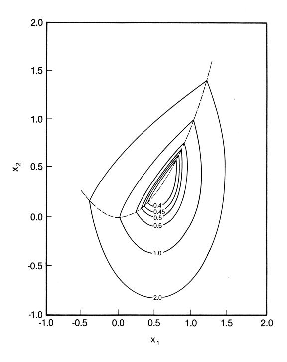
Fig. 3 Contours for the two-dimensional problem (5),  $f_1(\mathbf{x}) = (x_1 - 1)^2 + x^2_2$ ,  $f_2(\mathbf{x}) = x^2_1 - x_2$ .
