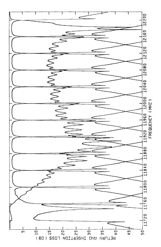
Fig. 6 Responses of the 12-channel multiplexer at the start of the optimization process.
