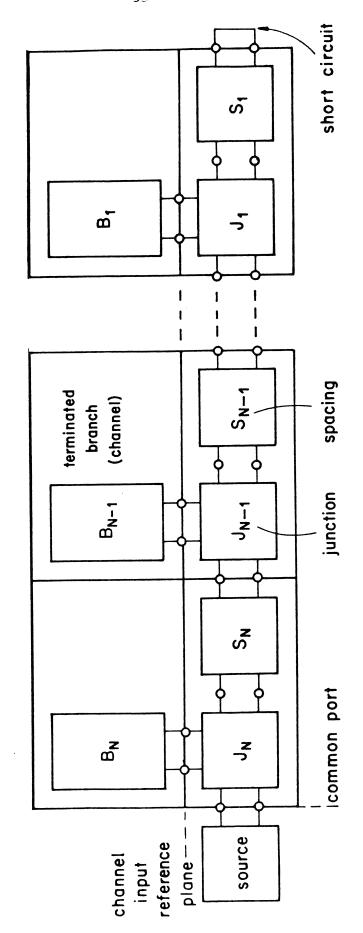
Fig. 5 The multiplexer configuration under consideration.  $J_1, J_2, \ldots, J_N$  are arbitrarily defined 3-port junctions,  $B_1, B_2, \ldots, B_N$  are terminated branches or channels which may each be represented in reduced cascade form and  $S_1, S_2, \ldots, S_N$  are usually waveguide spacing elements.
