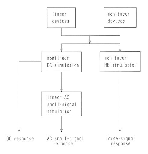
Fig. 1 Block diagram of logical connections among devices, simulators, and responses.
