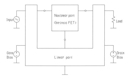
Fig. 2 A generic representation of a FET circuit for McCAE simulation.
