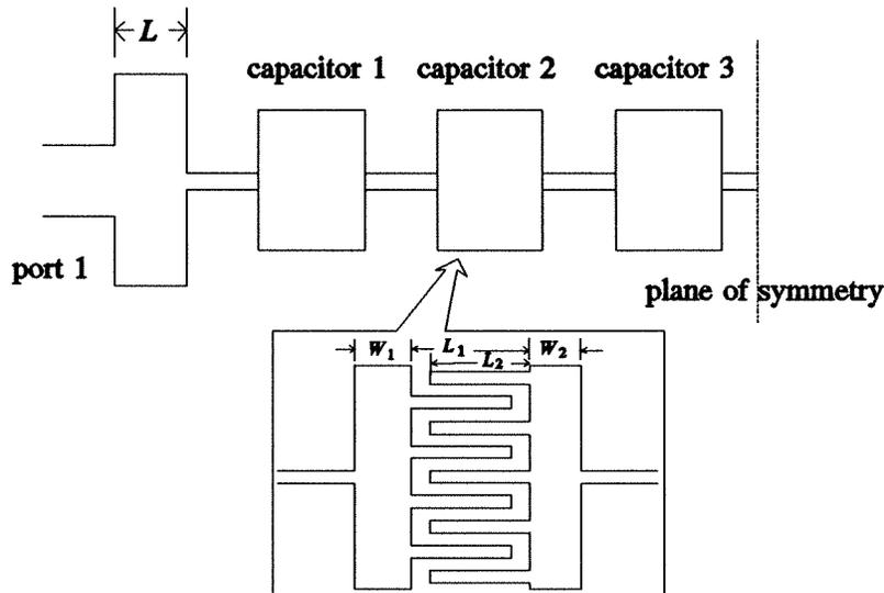
utilizes thin microstrip lines and interdigital capacitors to realize inductances and capacitances of a synthesized lumped ladder circuit
