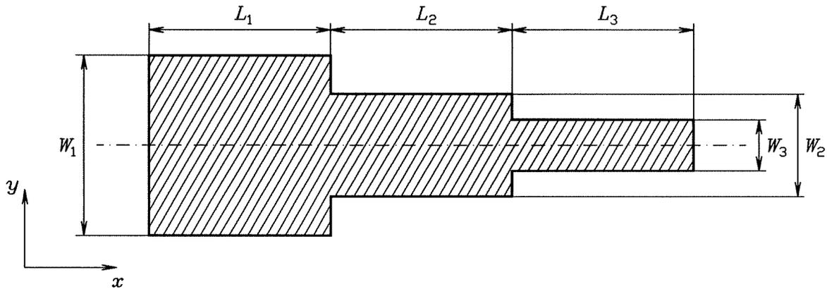
designed on a 0.635 mm thick substrate with relative dielectric constant of 9.7
