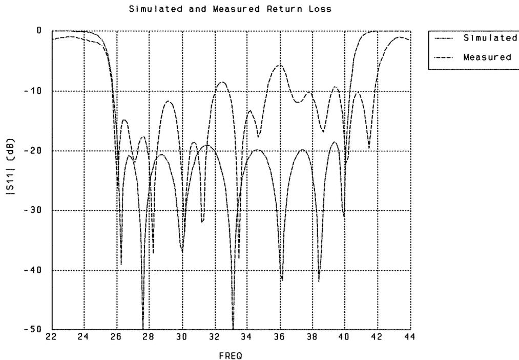
recent improvements in the field solver analysis of interdigital capacitors will improve the accuracy of the bandwidth prediction
