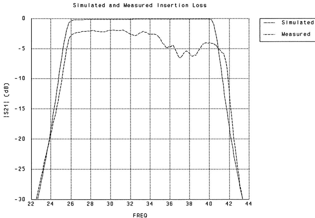
the insertion loss flatness will clearly improve after return loss has been tuned
