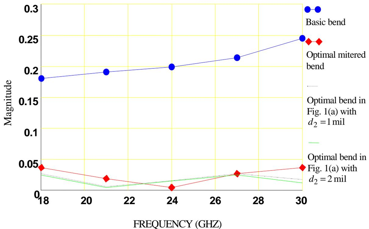
Fig. 5  $|S_{11}|$  for the basic 90° right angle microstrip bend and the optimal bends shown in Fig. 1 and Fig. 2
