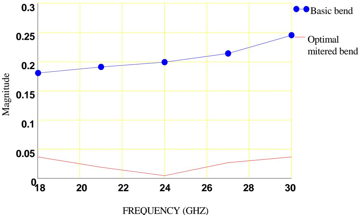
Fig. 3  $|S_{11}|$  for the basic 90° right angle microstrip bend and the optimal mitered bend in Fig. 1
