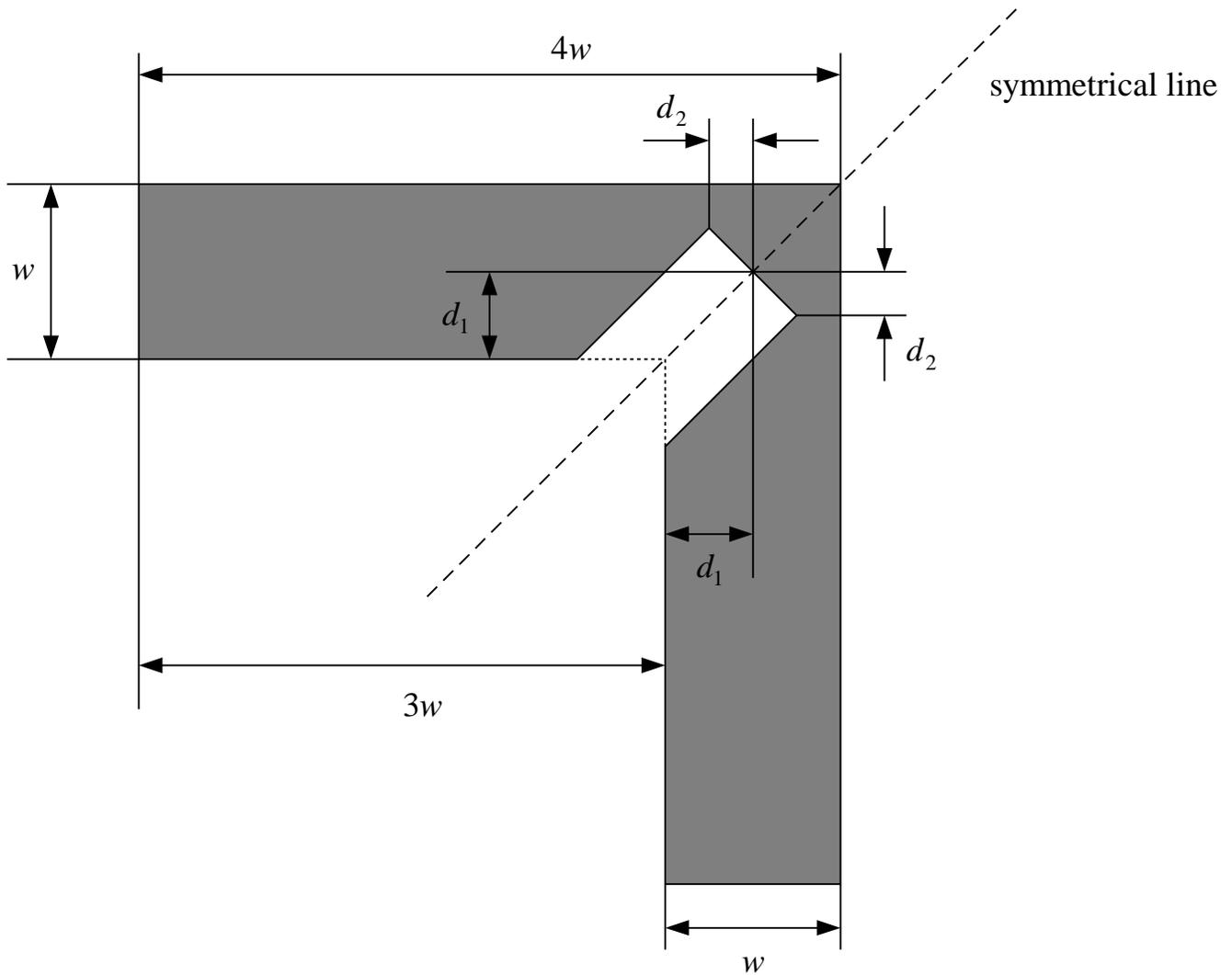
Fig. 2 a bend with a slit
