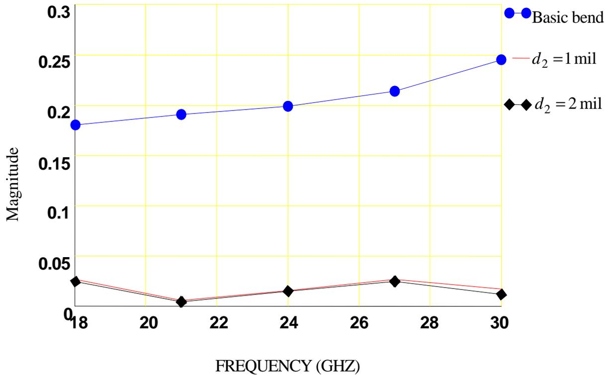
Fig. 4  $|S_{11}|$  for the basic 90° right angle microstrip bend and the optimal bend in Fig. 2 with  $d_2$  equal to 1mil and 2 mil
