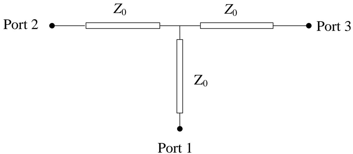
$$\begin{aligned} S_{11} = S_{22} = S_{33} &= \frac{V_1^-}{V_1^+} \Bigg|_{V_2^+ = V_3^+ = 0} = \frac{Z_L - Z_0}{Z_L + Z_0} \Bigg|_{Z_0 \text{ on ports 2 and 3}} \\ &= \frac{Z_0/2 - Z_0}{Z_0/2 + Z_0} = -\frac{1}{3} \end{aligned}$$
