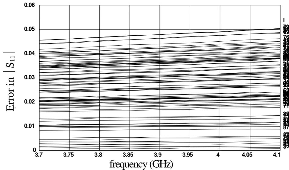
the difference in  $|S_{11}|$  computed by Sonnet *em* simulator and by Jansen empirical model after applying SMSM
