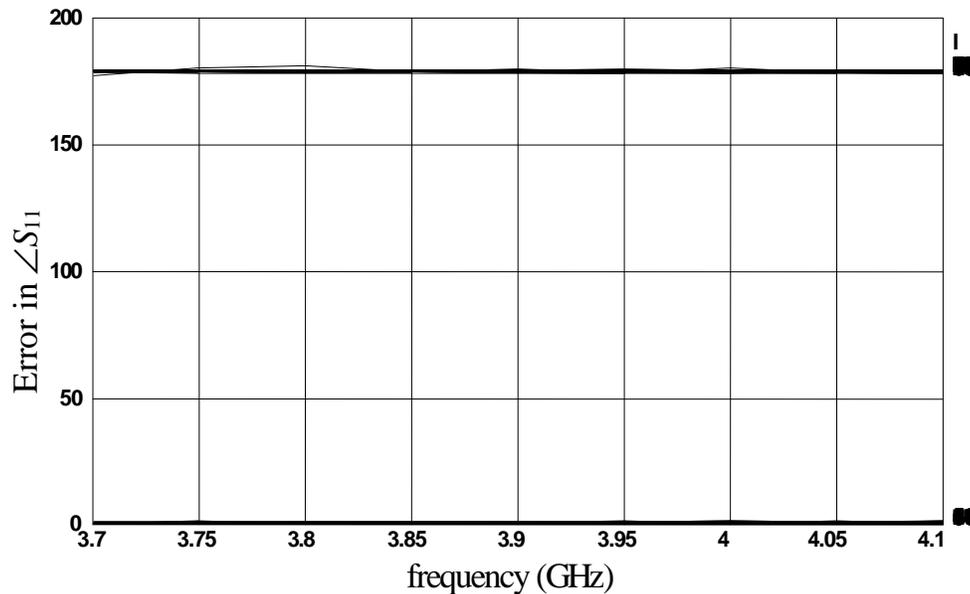
the difference in the phase of  $S_{11}$  computed by Sonnet *em* simulator and by Jansen empirical model after applying SMSM
