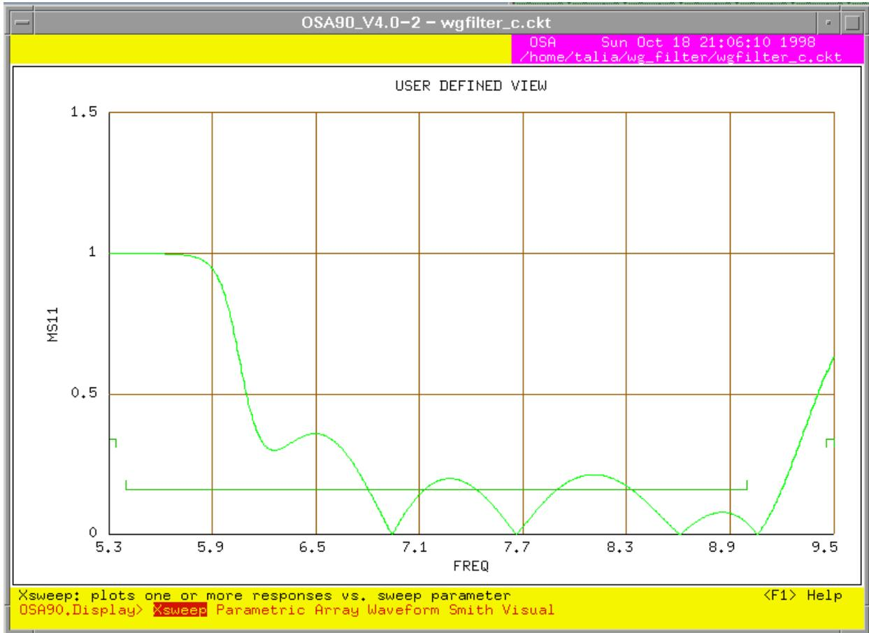
Fig. 9.  $|S_{11}|$  response of the coarse model before optimization.
