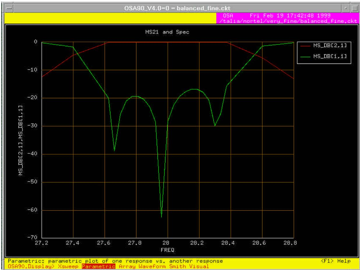
Fig. 12.  $|S_{21}|$  and  $|S_{11}|$  responses in dB of the fine model of the balanced filter after the optimization is completed.
