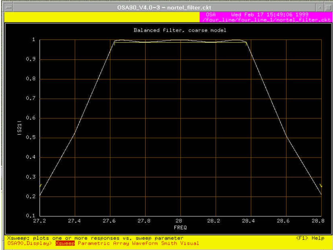
Fig. 7.  $|S_{21}|$  response of the refined coarse model after optimization.
