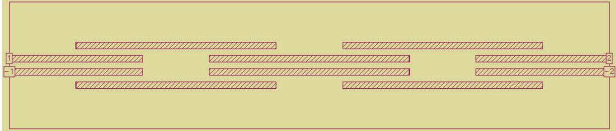
Fig. 8. Nominal project for geometry capture of the microstrip balanced filter structure with Empipe.
