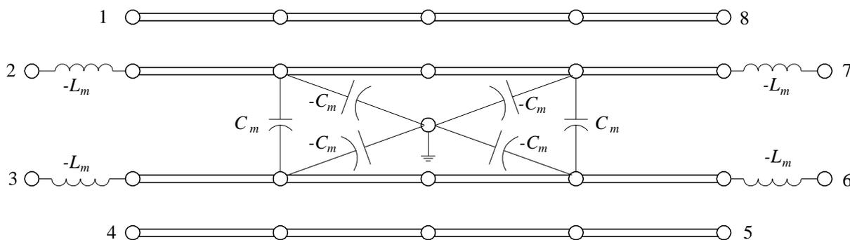
Fig. 3. The equivalent circuit used as a very coarse approximation of the odd mode of a section of two coupled coupled-microstrip lines.
