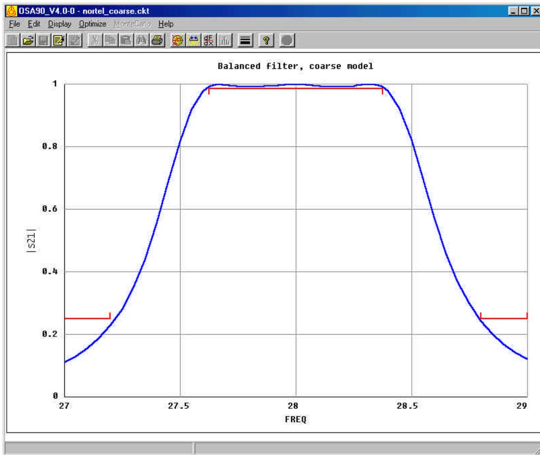
Fig. 5.  $|S_{21}|$  response of the coarse model after the minimax optimization.
