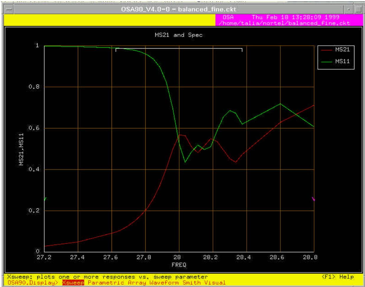
Fig. 10.  $|S_{21}|$  and  $|S_{11}|$  responses of the fine model of the balanced filter at the starting point of optimization.
