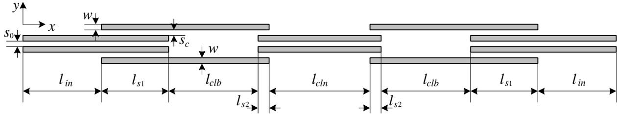
Fig. 1. The balanced microstrip filter: general geometry and parameter notation.
