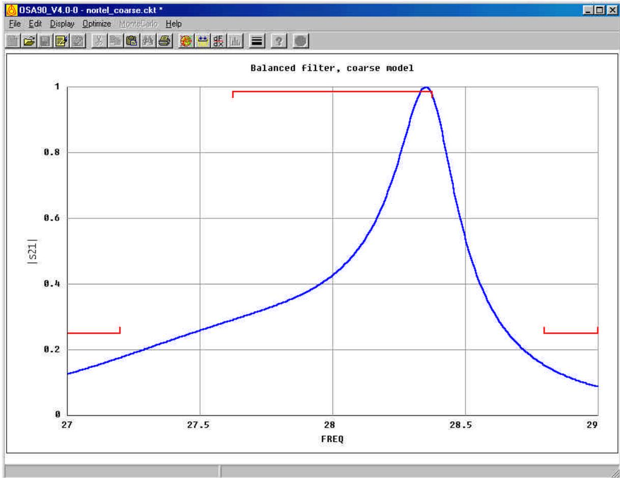
Fig. 4. The coarse model  $|S_{21}|$  response at the starting point (the nominal values).
