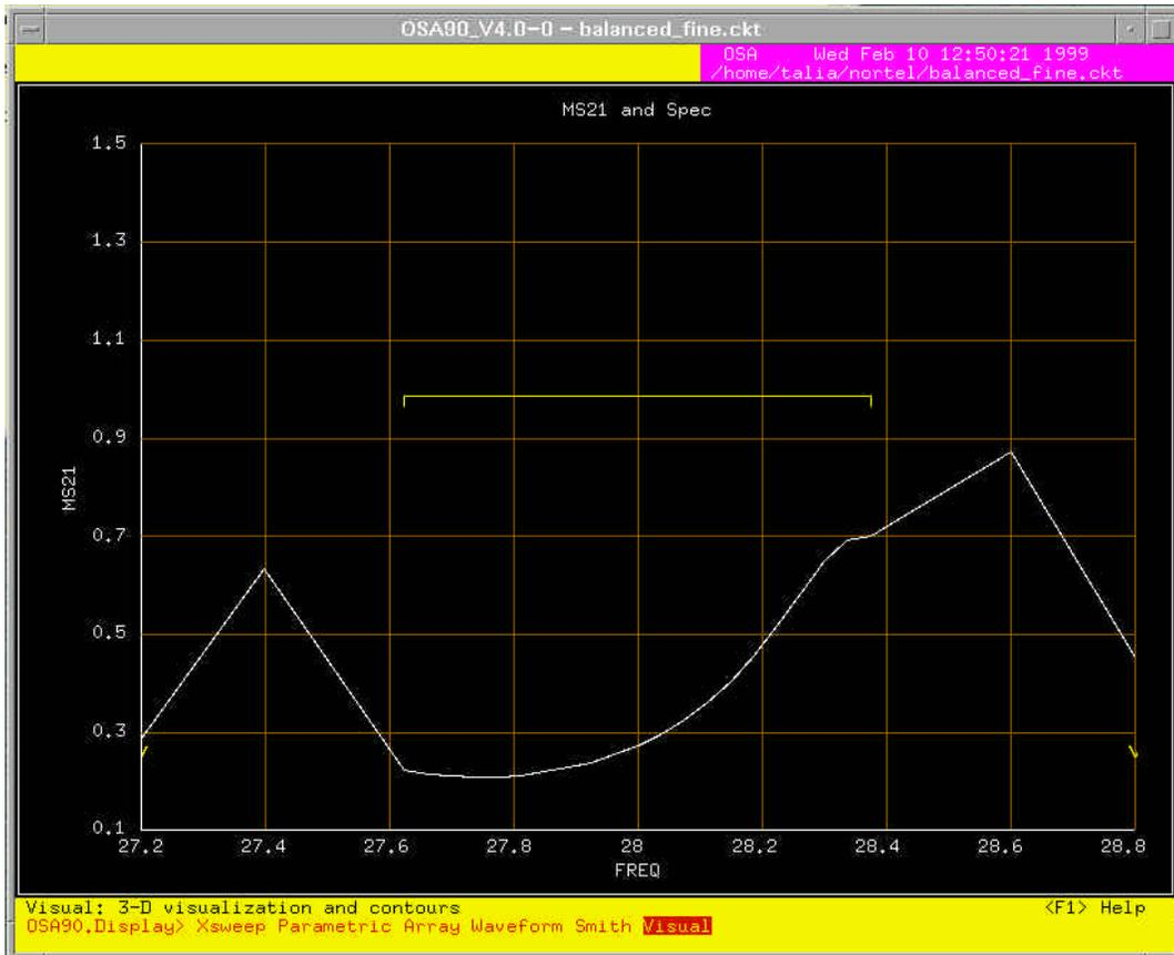
Fig. 2. The fine model  $|S_{21}|$  response for the nominal set of parameters.
