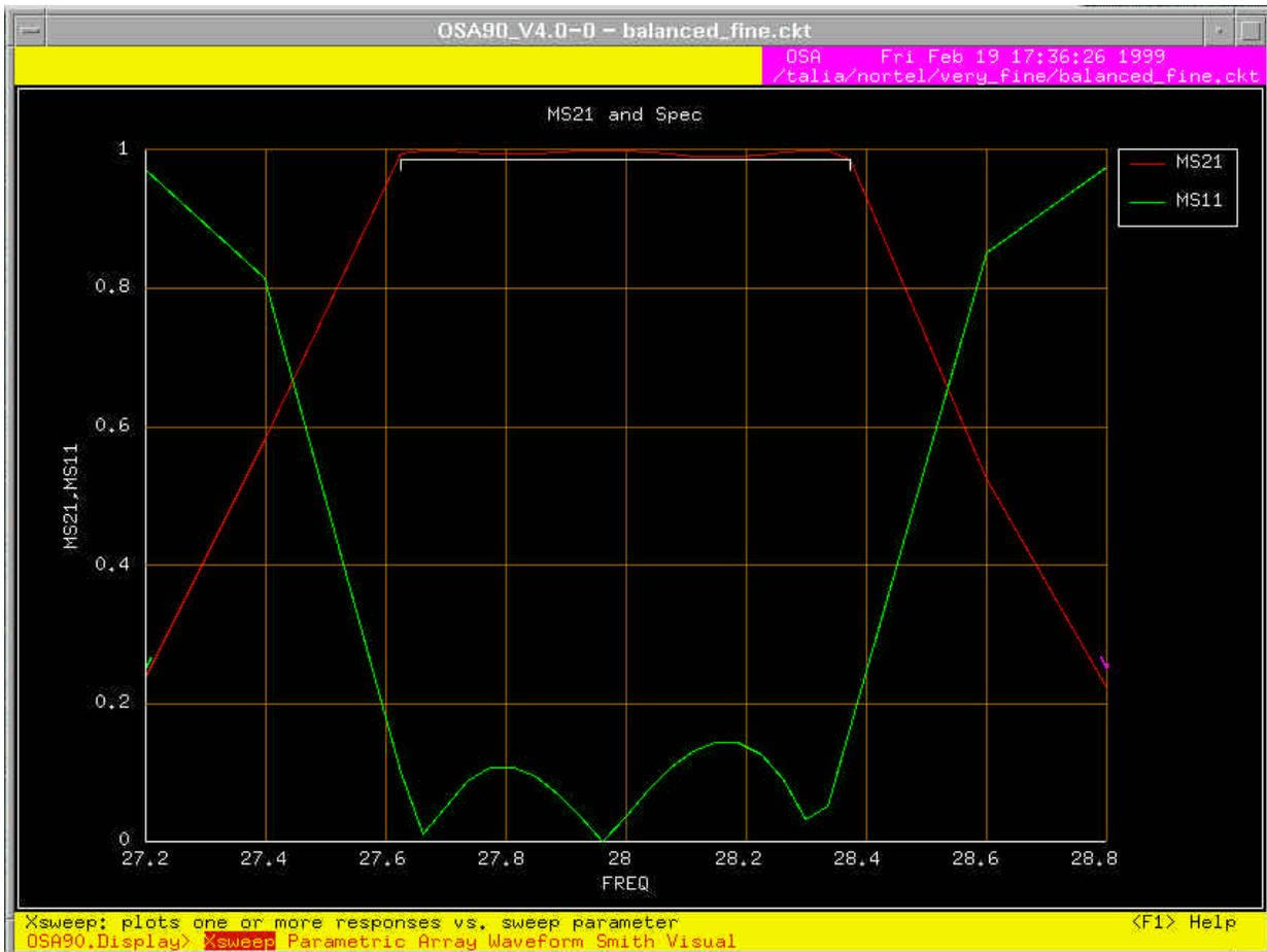
Fig. 11.  $|S_{21}|$  and  $|S_{11}|$  responses of the fine model of the balanced filter after the optimization is completed.
