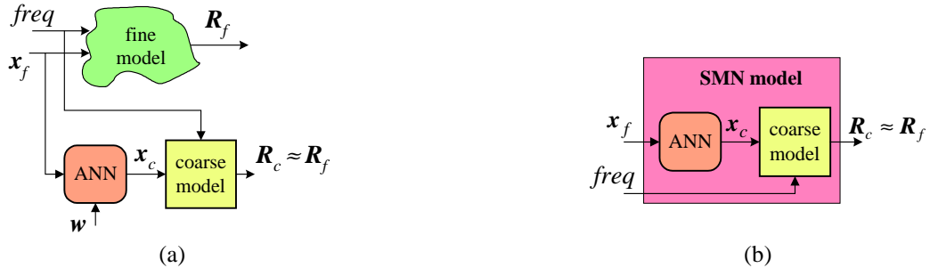
Fig. 2. Space-Mapped Neuromodeling concept: (a) SM neuromodeling, (b) SMN model.
