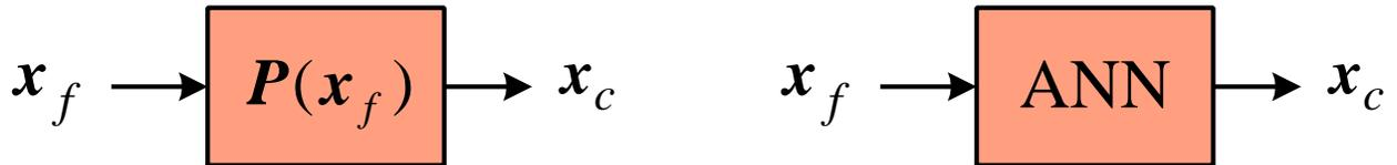
using a three layer perceptron (3LP)
