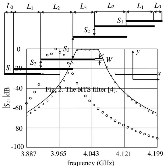
Fig. 3. Results for the HTS filter; The optimal coarse response (—), the initial fine response (o) and the final fine model design ( $\diamond$ ).
