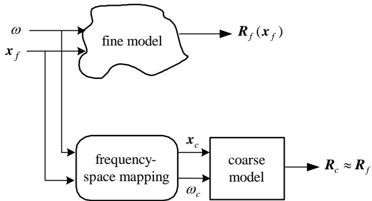
Fig. 1. The Frequency-Space Mapping Super Model (FSMSM) concept.
