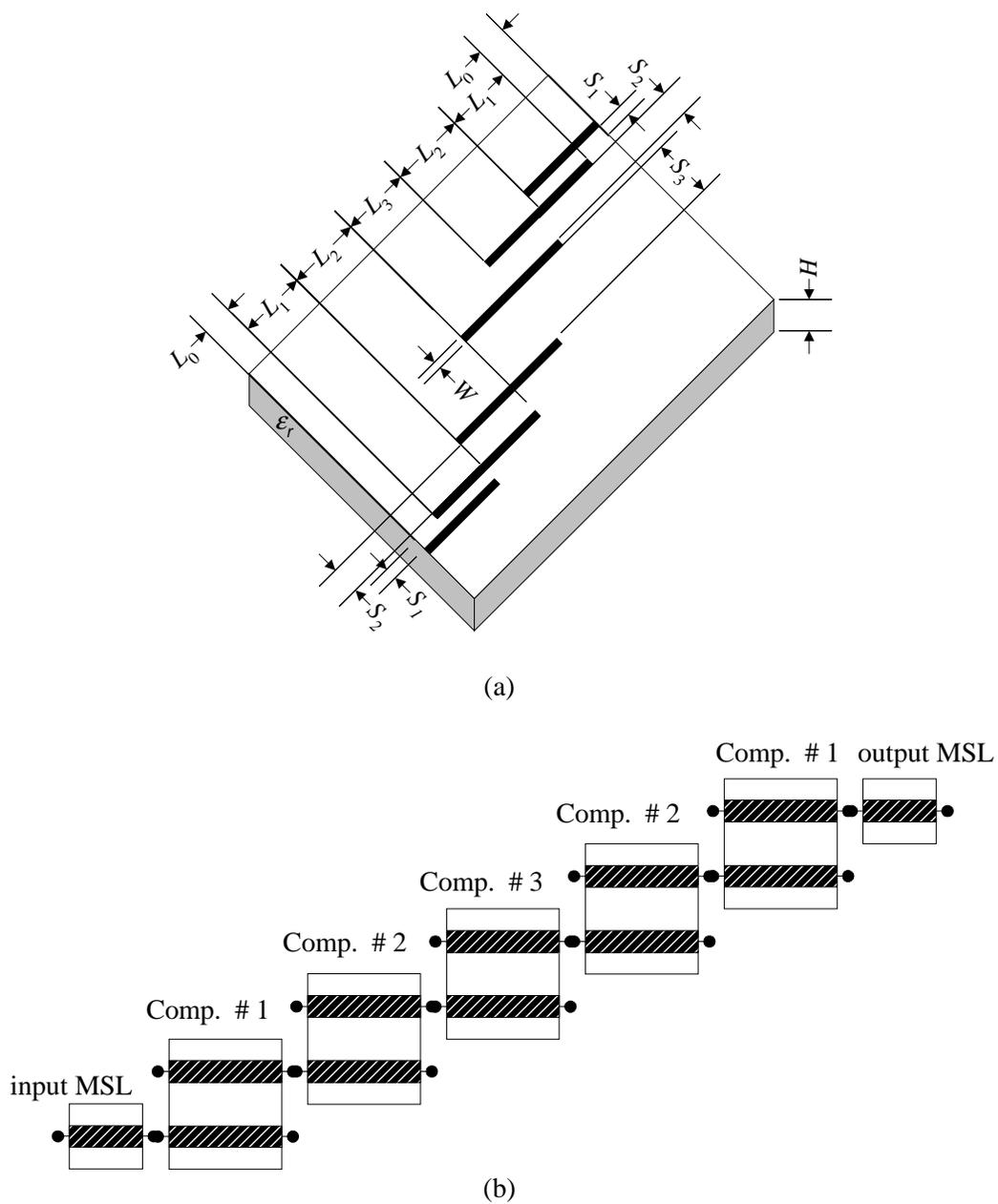
Fig. 6. The HTS filter: (a) the physical structure; (b) the coarse model.
