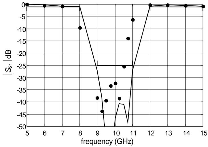
Fig. 13. The fine model response (••) versus the coarse model response (—) of the open stub filter at the initial solution.
