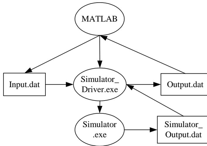
Fig. 3. Driving EM/circuit simulators from inside Matlab.
