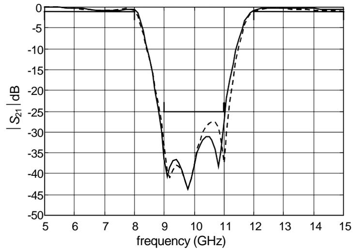
Fig. 15. The fine model responses of the open stub filter at the solution obtained by direct Momentum optimization (—) and by our ESMDF algorithm (----).
