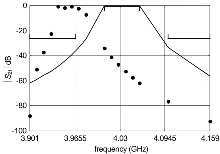
Fig. 8. The Sonnet *em* fine model response (●●) and the coarse model response (—) of the HTS filter at the initial solution.
