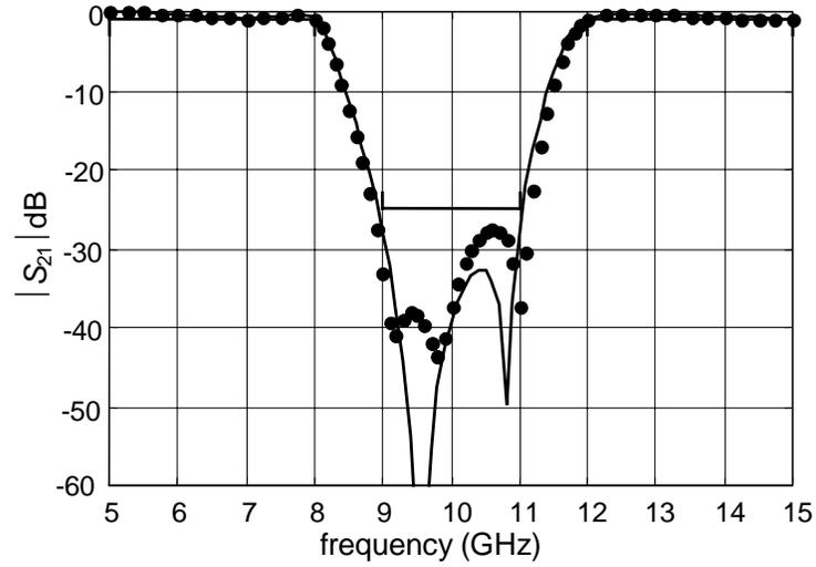
Fig. 14. Detailed frequency sweep of the fine and coarse model responses of the open stub filter at the final solution.
