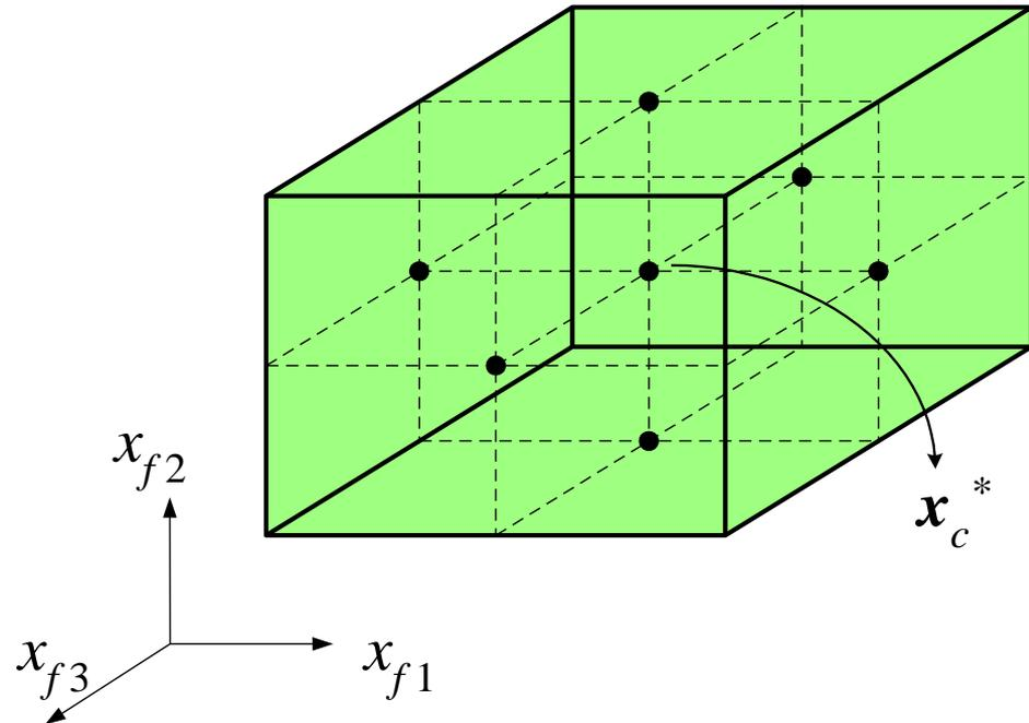
( $2n + 1$  learning base points for a microwave circuit with  $n$  design parameters)
