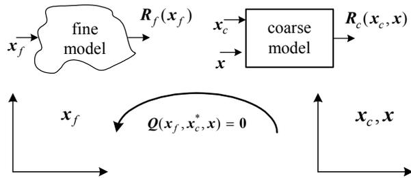
Fig. 4. Illustration of Implicit Space Mapping (ISM)—optimization.
