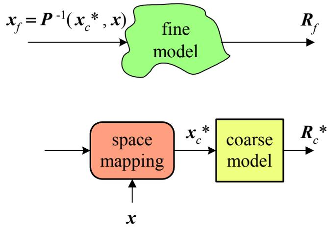
Fig. 10. Explicit mapping—verification of the fine model.
