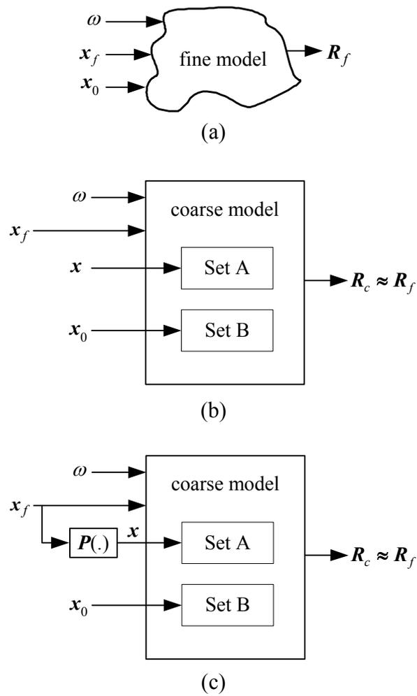
Fig. 17. Calibrating (optimizing) the preassigned parameters  $x$  in Set A results in aligning the coarse model (b) or (c) with the fine model (a). In (c) we illustrate the ESMDF approach [5], where  $\mathbf{P}(\cdot)$  is a mapping from optimizable design parameters to preassigned parameters.
