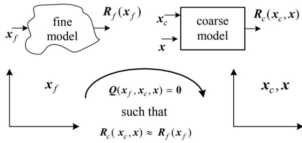
Fig. 3. Illustration of Implicit Space Mapping (ISM)—modeling.
