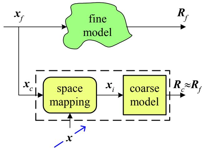
Fig. 13. Implicit mapping—Parameter Extraction w.r.t. preassigned parameters.
