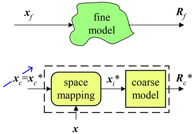
Fig. 11. Implicit mapping—optimization of the mapped coarse model.
