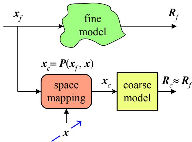
Fig. 8. Explicit mapping—Parameter Extraction.
