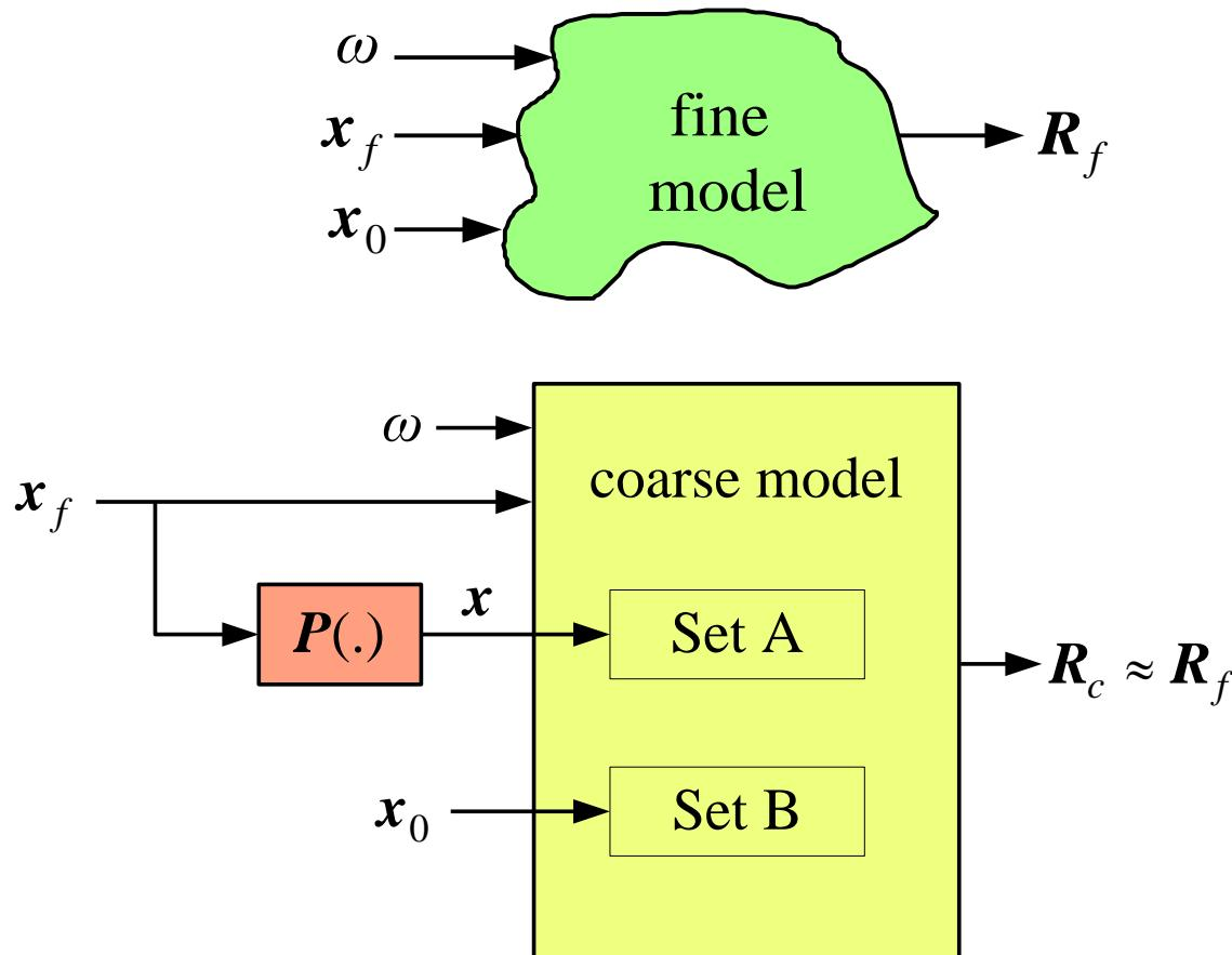
Key Preassigned Parameters (KPP) (ESMDF algorithm)
