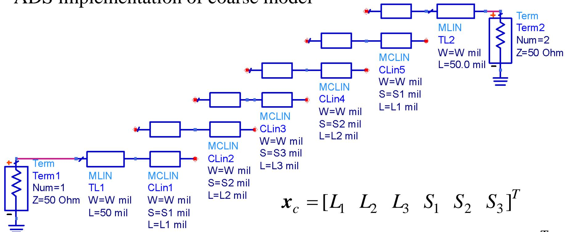
$$\boldsymbol{x}_c = [L_1 \quad L_2 \quad L_3 \quad S_1 \quad S_2 \quad S_3]^T$$
