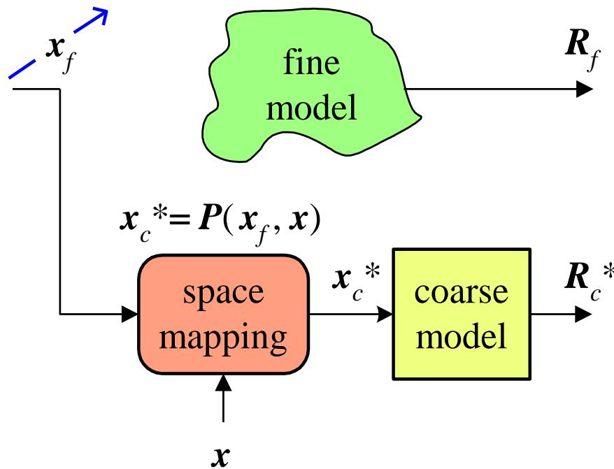
find the  $x_f$  corresponding to the optimal coarse space parameters
