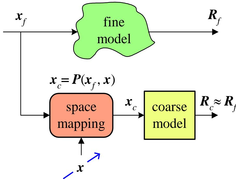
set up the mapping and parameter extract
