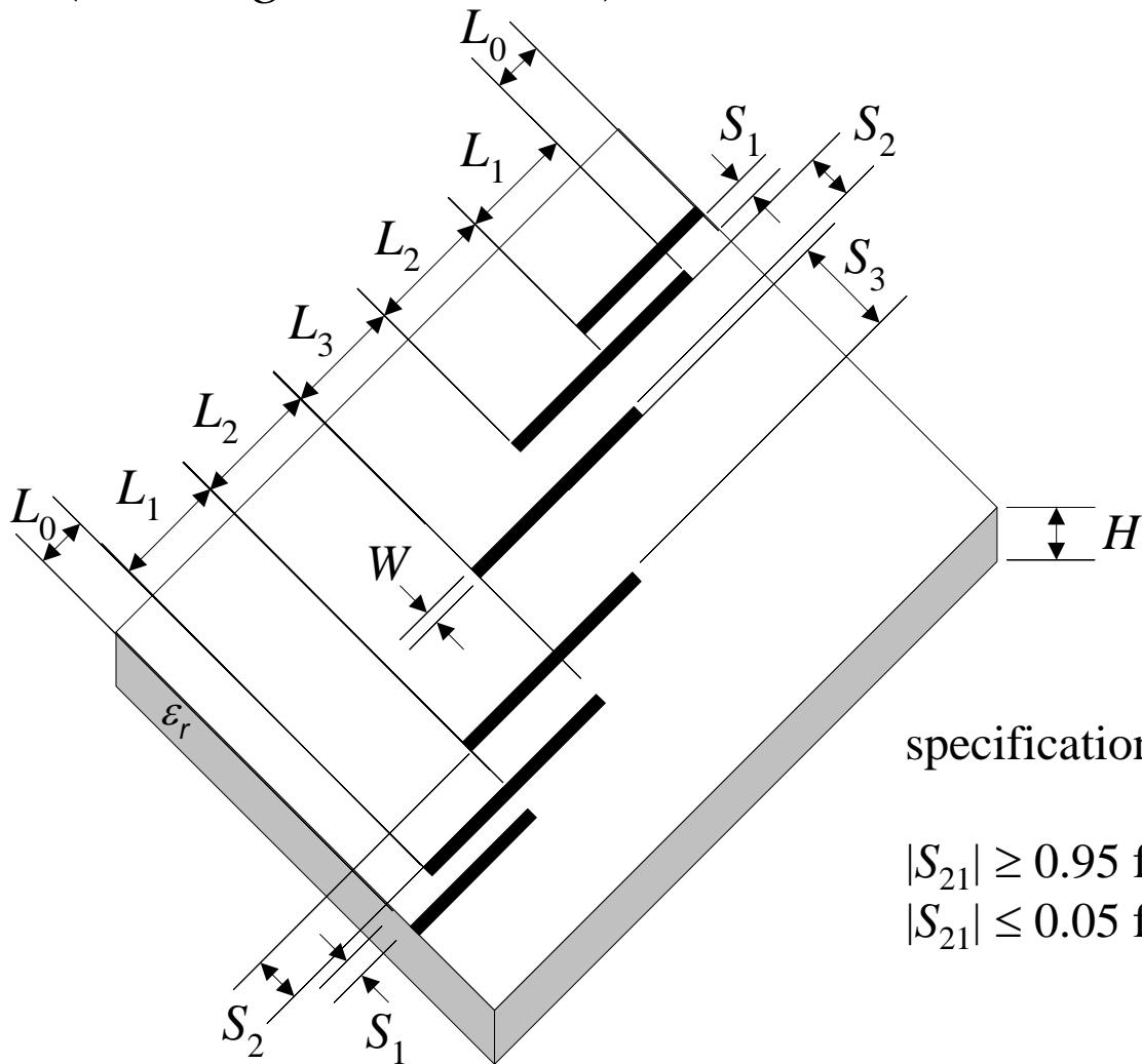
we take  $L_0 = 50$  mil,  $H = 20$  mil,  $W = 7$  mil,  $\epsilon_r = 23.425$ , loss tangent =  $3 \times 10^{-5}$ ; the metalization is considered lossless
