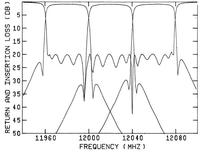
Fig. 4 Responses of the multiplexer at the solution.
