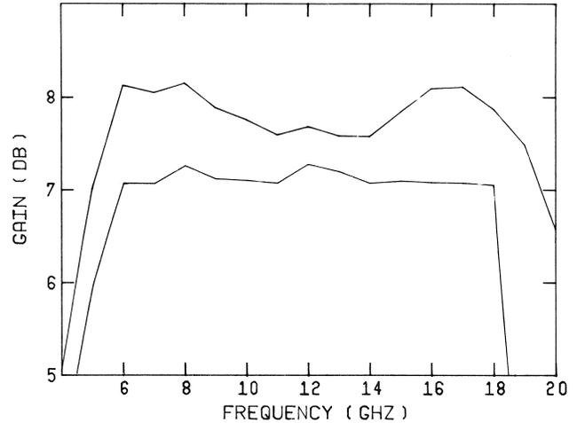
Fig. 2 The worst-case envelope for the amplifier response.
