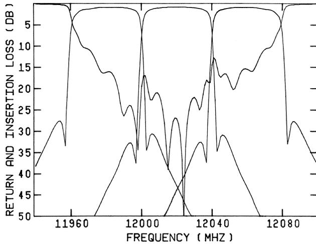
Fig. 3 Responses of the multiplexer at the starting point.
