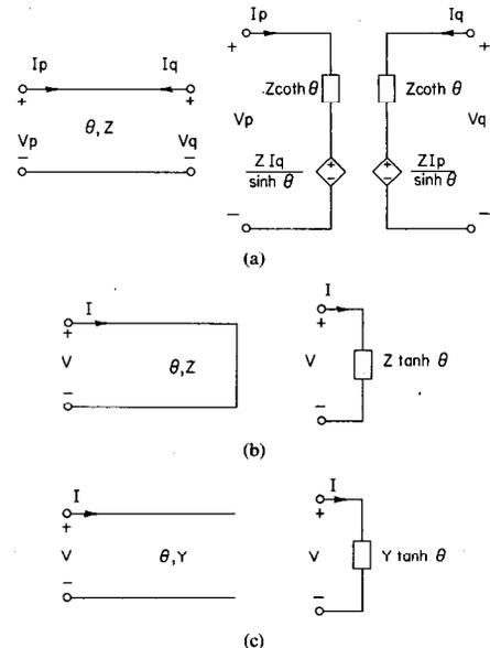
Fig. 1. Uniformly distributed elements with convenient representations. (a) Uniform line. (b) Short-circuited line. (c) Open-circuited line.
