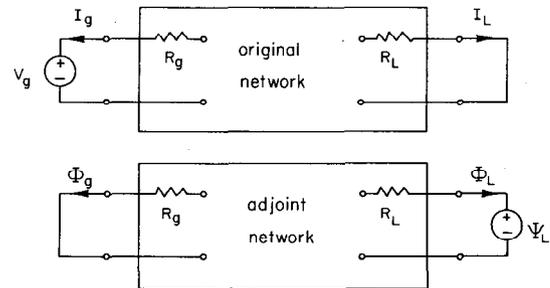
Fig. 2. Network for insertion loss design.
