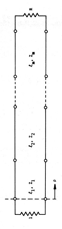
$l_{q}$  =7.49481 cm is the quarter-wavelength at center frequency. 3-section:  $\ell_1 = \ell_2 = \ell_3 = \ell_q$ ,  $Z_1 = 1.63471$ ,  $Z_2 = 3.16228$ ,  $Z_3 = 6.11729$ . m-section resistively terminated cascade of transmission Optimum matching over 100% band centered at 1GHz for R=10 occurs for the following parameter values. 2-section:  $\ell_1 = \ell_2 = \ell_q$ ,  $z_1 = 2.23605$ ,  $z_2 = 4.4721$ lines. Figure 1
