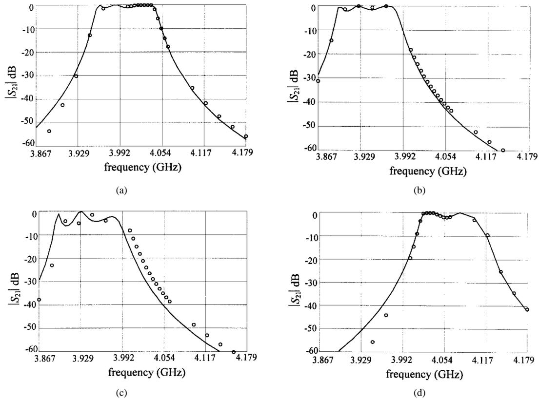
Fig. 15. The fine-model response (o) and the corresponding coarse-model response (—): (a) at the first point, (b) at the second point, (c) at the third point, and (d) at the fourth point utilized in the four-point parameter extraction for the HTS filter. Note that only points in the range from 3.967 to 4.099 GHz were actually used.
