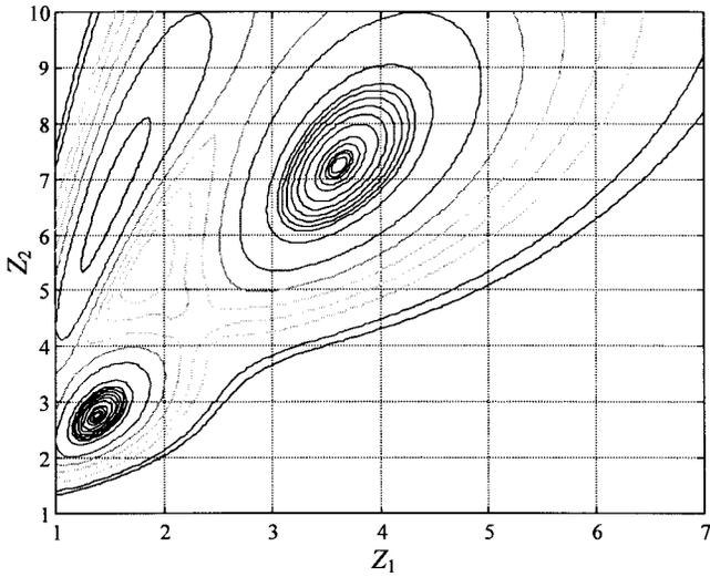
Fig. 6. The contours of  $Q(\mathbf{x}, V^{(1)})$  for the 10:1 impedance transformer.
