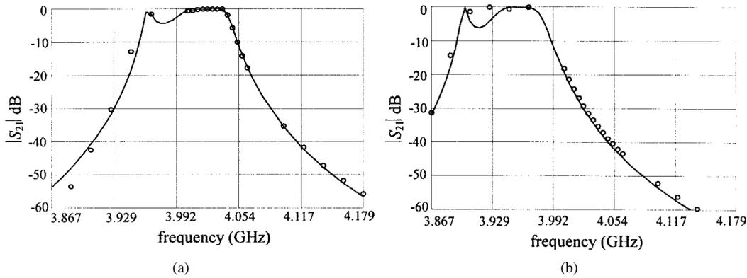
Fig. 13. The fine-model response (o) and the corresponding coarse-model response (—): (a) at the first point and (b) at the second point utilized in the DPE for the HTS filter. Note that only points in the range from 3.967 to 4.099 GHz were actually used.
