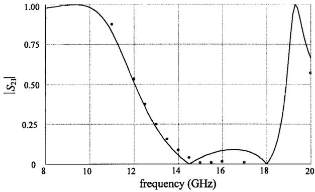
Fig. 18. The fine-model response (o) and the corresponding coarse-model response (—) at the point  $\mathbf{x}_{os}^{e(1)}$  for the DFS filter.
