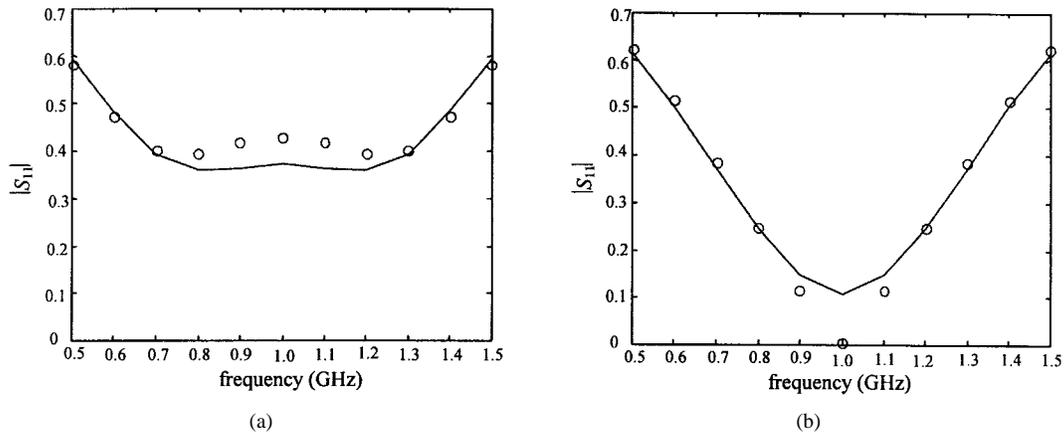
Fig. 7. The fine-model response (o) and the corresponding coarse-model response (—): (a) at the first point and (b) at the second point utilized in the DPE for the 10:1 impedance transformer.
