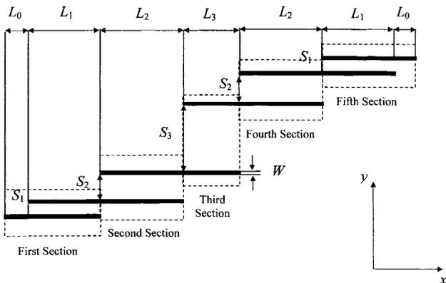
Fig. 11. The HTS filter [9].
