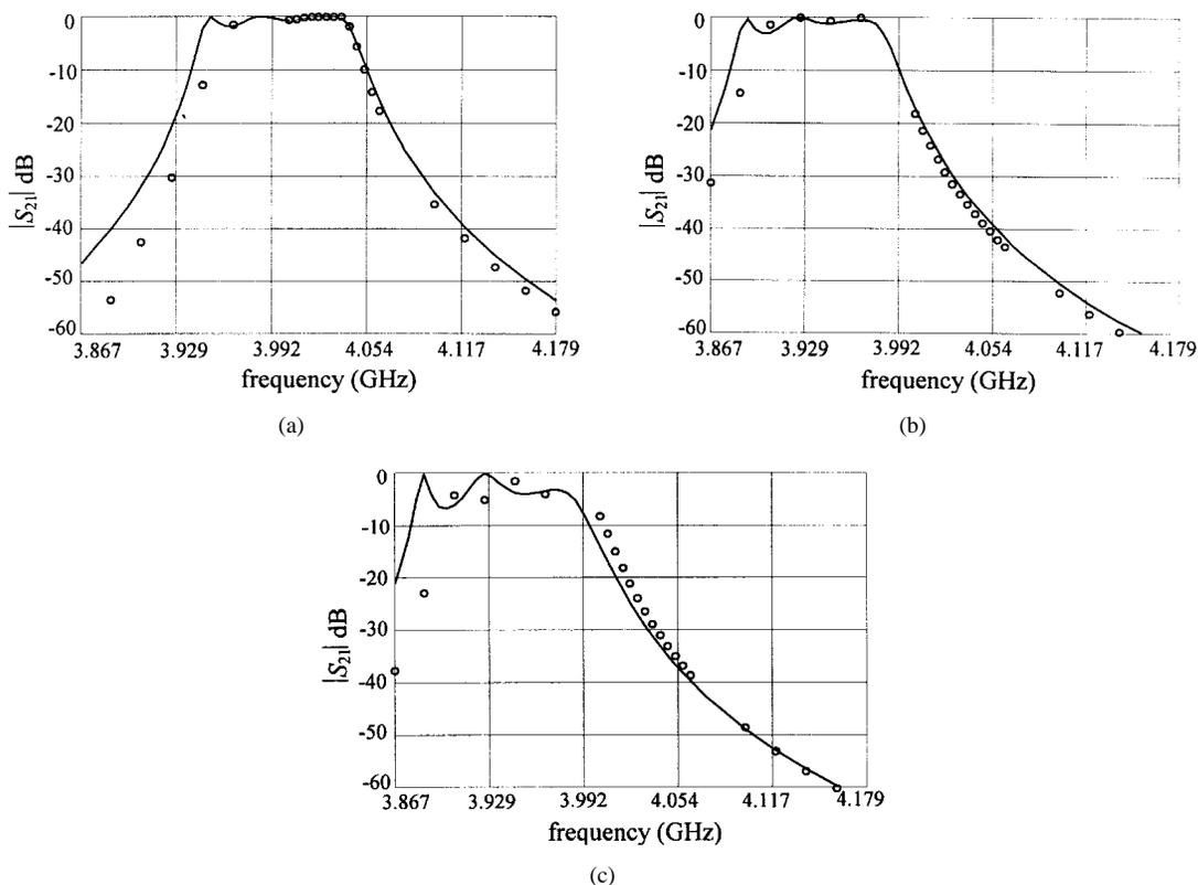
Fig. 14. The fine-model response (o) and the corresponding coarse-model response (—): (a) at the first point, (b) at the second point, and (c) at the third point utilized in the three-point parameter extraction for the HTS filter. Note that only points in the range from 3.967 to 4.099 GHz were actually used.
