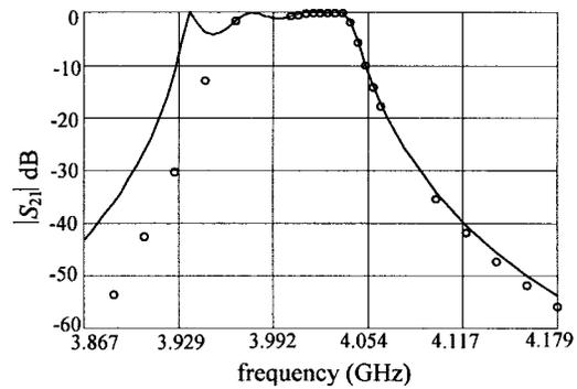
Fig. 12. The fine-model response (o) and the corresponding coarse-model response (—) at the point utilized in the SPE for the HTS filter. Note that only points in the range from 3.967 to 4.099 GHz were actually used.
