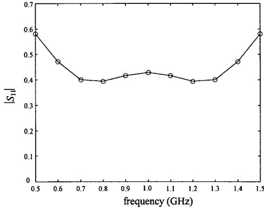
Fig. 5. The responses of the given fine-model point (o) and the coarse-model response (—) at the point  $\mathbf{x}_{os}^{e(1)}$  for the 10:1 impedance transformer.
