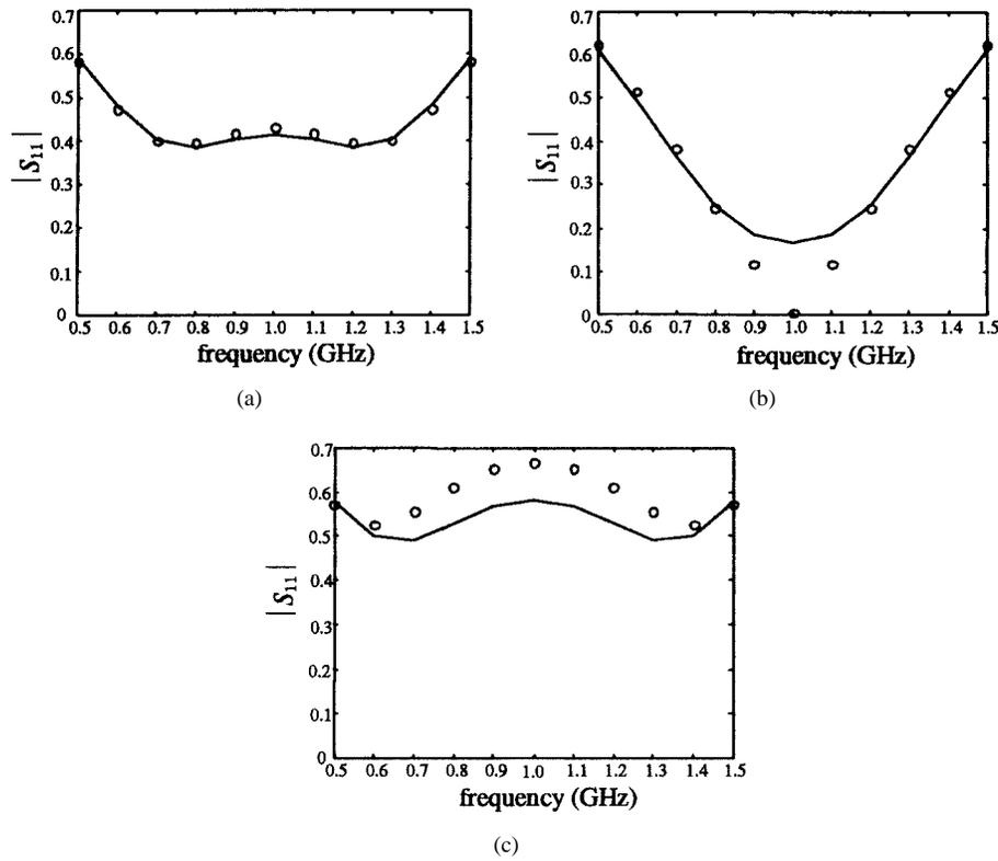
Fig. 9. The fine-model response (o) and the corresponding coarse-model response (—): (a) at the first point, (b) at the second point, and (c) at the third point utilized in the three-point parameter extraction for the 10:1 impedance transformer.
