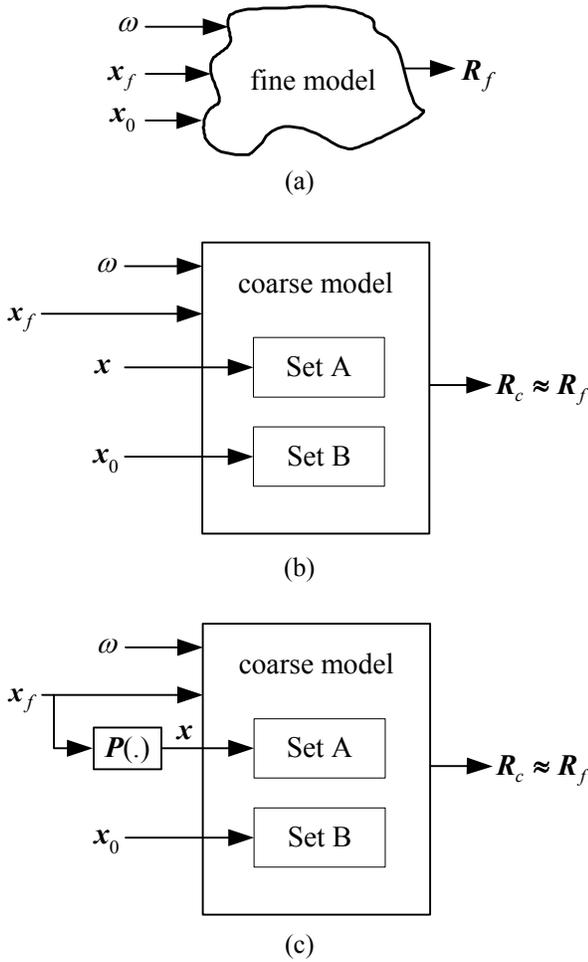
Fig. 2. Calibrating (optimizing) the preassigned parameters  $x$  in Set A results in aligning the coarse model (b) or (c) with the fine model (a). In (c) we illustrate the ESMDF approach [5], where  $P(\cdot)$  is a mapping from optimizable design parameters to preassigned parameters.
