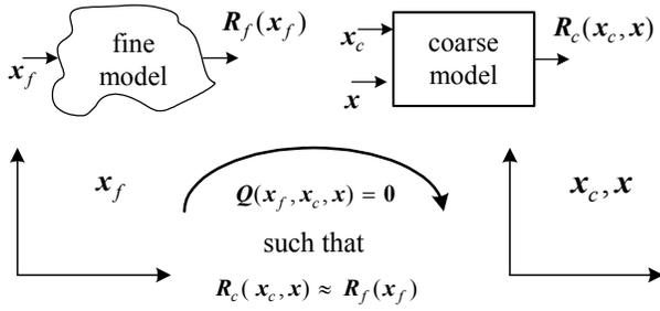
Fig. 1. Illustration of Implicit Space Mapping (ISM).
