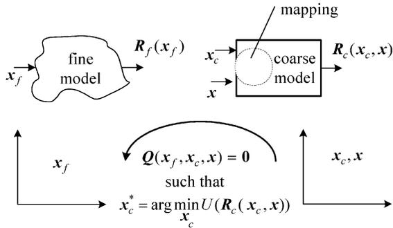
Fig. 4. Illustration of ISM prediction. Here,  $Q = 0$  is solved for  $\mathbf{x}_c^*$ .
