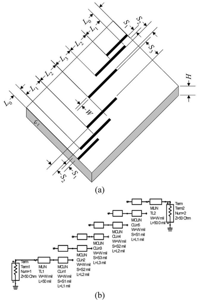
Fig. 10. HTS filter [17]. (a) Physical structure and (b) coarse model as implemented in Agilent ADS.
