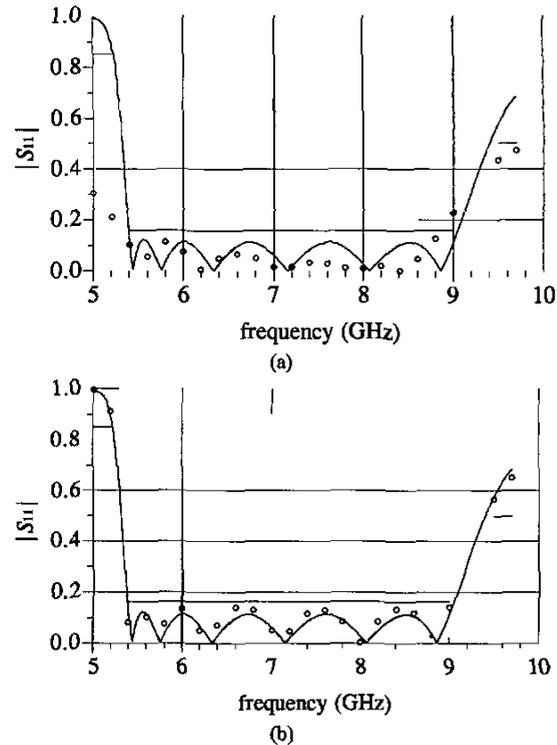
Fig. 7. H-plane filter optimal coarse model response (—), and the fine model response at: (a) initial solution (o); (b) solution reached via RRSM after 4 iterations (o).
