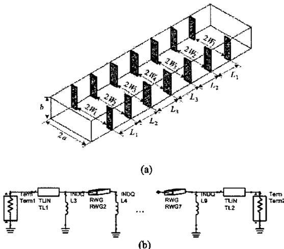
Fig. 6. (a) Six-section H-plane waveguide filter (b) ADS coarse model.
