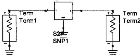
Fig. 5. S2P (2-Port S-Parameter File) symbol with terminals.
