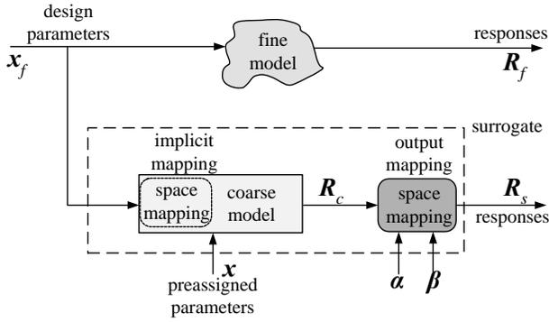
Fig. 1. The implicit and output SM concepts [10]. We calibrate the surrogate against the fine model utilizing the preassigned parameters  $\mathbf{x}$ , e.g., dielectric constant, and the output response mapping parameters: the scaling matrix  $\alpha$  and the shifting vector  $\beta$ .
