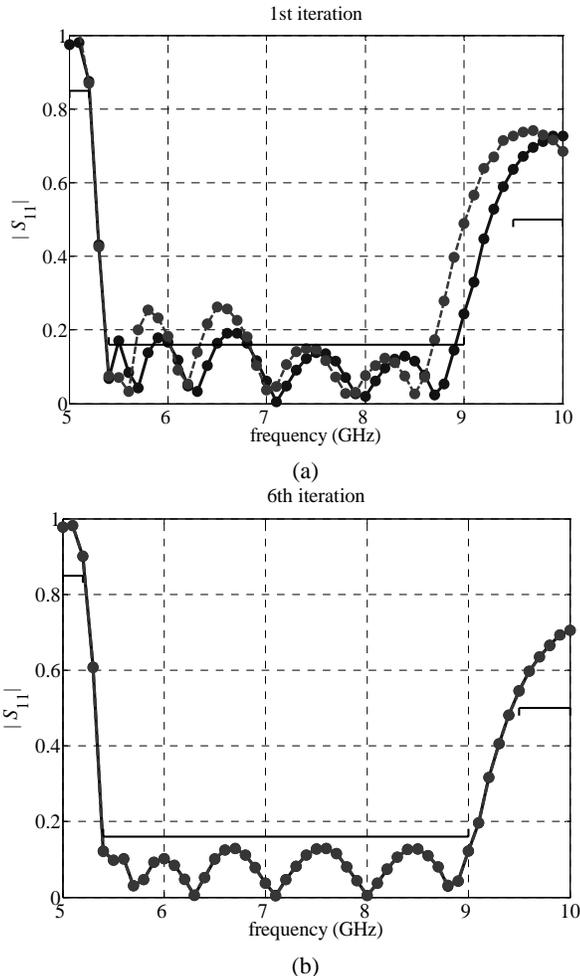
Fig. 3. The surrogate response (---●---) and the corresponding fine model response (—●—) at: (a) the initial design, and (b) the final design for the six-section H-plane waveguide filter designed using the coarse-grid MEFiSTo model.
