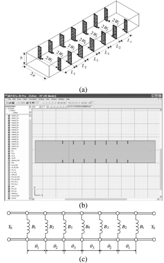
Fig. 2. The six-section H-plane waveguide filter: (a) the 3D view [10]. (b) MEFiSTo snapshot of the cross section. (c) the equivalent empirical circuit model [10].
