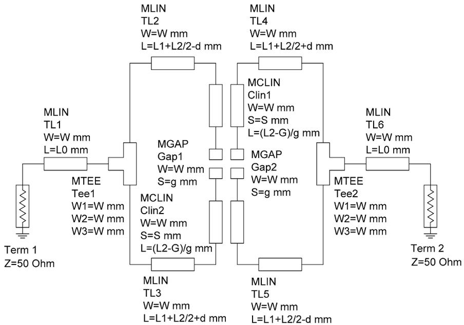
**Fig. 7** Coarse model of the bandpass filter with two transmission zeros (Agilent ADS)
