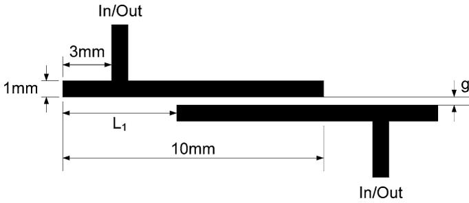
**Fig. 1** Geometry of the second-order tapped-line microstrip filter (Manchec et al. 2006)
