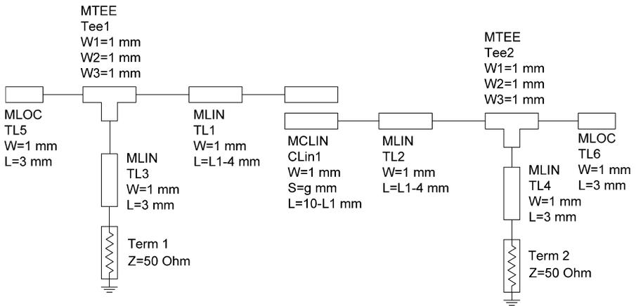
**Fig. 2** Coarse model of the second-order tapped-line microstrip filter (Agilent ADS)
