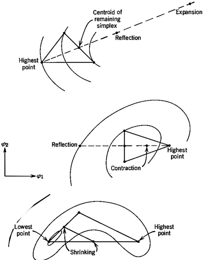
FIGURE 6-15 Examples of moves made by the simplex method.
