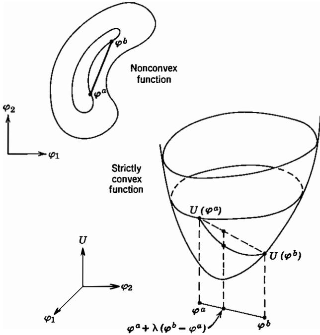
FIGURE 6-3 Illustration of convexity.
