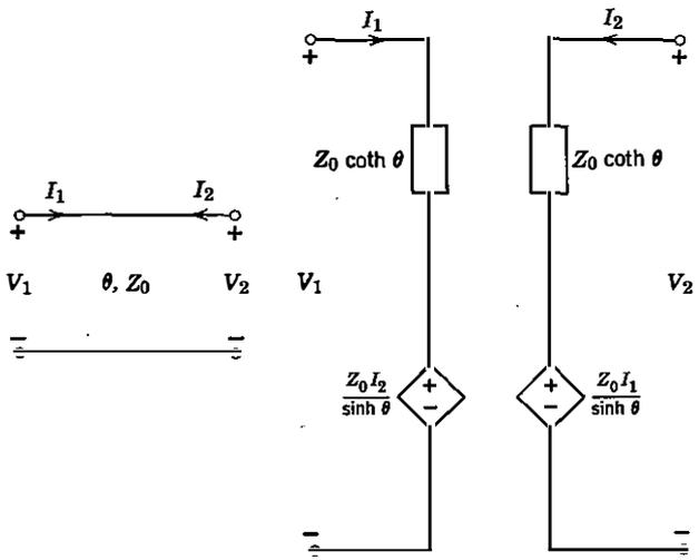
FIGURE 6-25 Uniform line and convenient representation.
