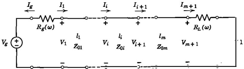
**FIGURE 6-9** Cascaded transmission-line filter between frequency-variable resistors.
