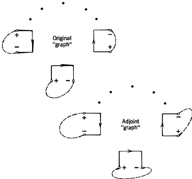
FIGURE 6-22 Representation of the elements of Figure 6-21 for application of Tellegen's theorem. Some  $i$ th equivalent branch might consist of an impedance  $z_{ii}$  in series with voltage generators of value  $z_{ij}I_j$ ,  $j = 1, 2, \dots$ . See, for example, Figure 6-25.
