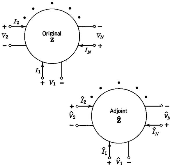
**FIGURE 6-21** Original and adjoint elements represented by impedance matrices. In general, many such elements suitably connected form the original and adjoint networks.
