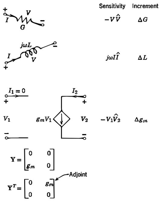
FIGURE 6-24 Sensitivities for three common elements: a resistor of conductance  $G$ , an inductor of inductance  $L$  and a voltage-controlled current source with transfer conductance  $g_m$ .
