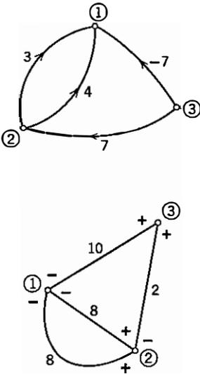
FIGURE 6-20 Illustration of Tellegen's theorem applied to two networks of the same topology. Observe that
